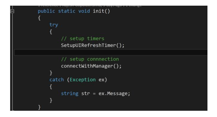
The function provides a connect method to establish a connection with Logi Options and also a timer that is used to demonstrate a simple use case of crown messages.
